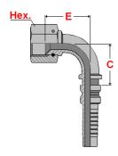
According to ISO 12151-5 and ISO 8434-2 According to SAE J516 / SAE J514
