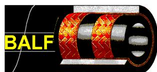
**Inner tube:** seamless oil resistant synthetic rubber
